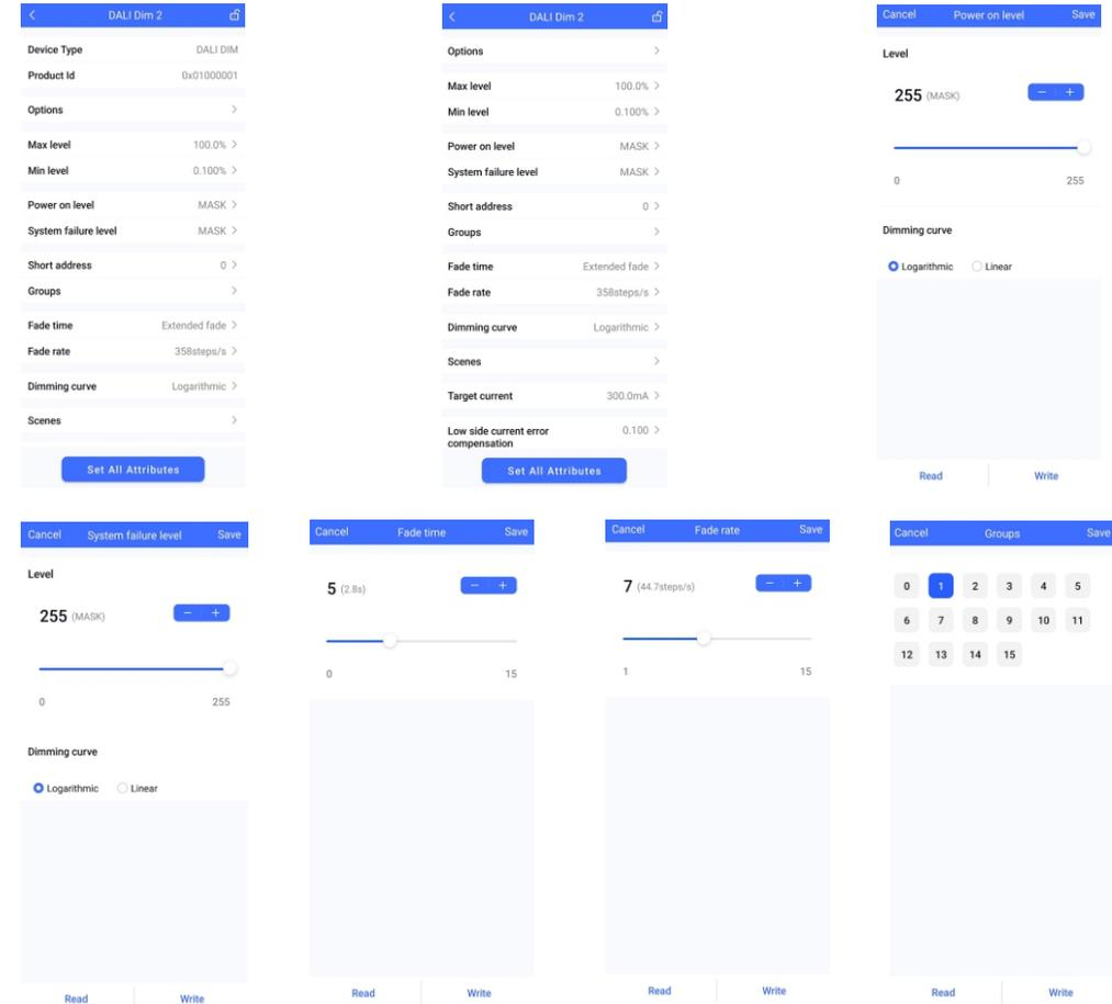
**Step 5: After setting, please save the selected configuration via NFC and power on the device.**
