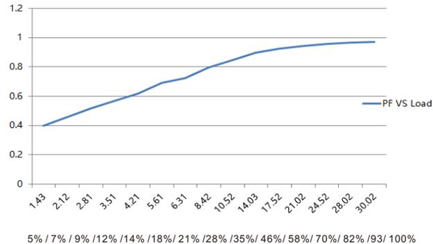
Note: Test data under 700mA gear
