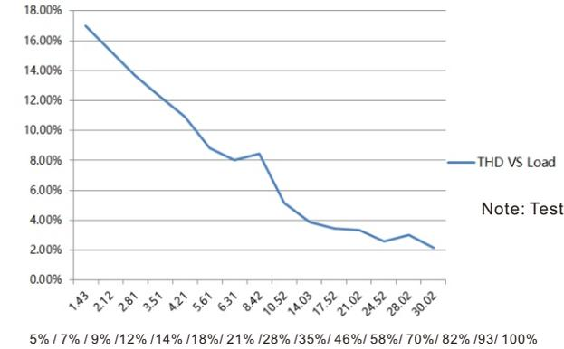
Note: Test data under 700mA gear
