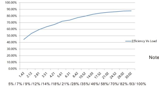
Note: Test data under 700mA gear
